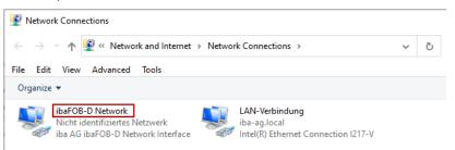
This network connection is required in 32Mbit Flex mode to communicate via TCP/IP with other Flex devices that are also connected via an ibaFOB-D board. There is only one network connection for all ibaFOB-D boards installed in an ibaPDA computer.
