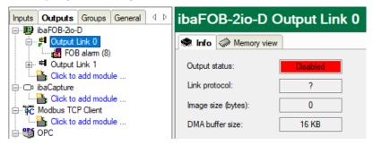
After the FOB alarm modules have been added the output signals (analog and/or digital) must be configured for each module.
