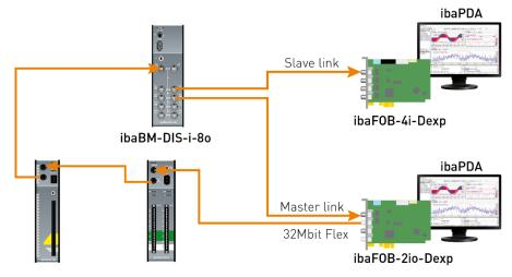
The example above with ibaBM-DIS-i-80 is similar to the example with ibaBM-FOX-i-30-D. The ibaBM-DIS-i-80 device mode must be set to copy mode (S1 = 0).
