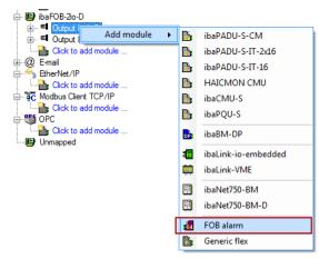
You can change the name of the FOB alarm module according to your needs. This provides the advantage of a clear assignment within the measuring system.
