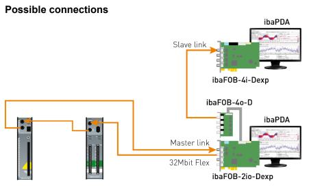
The data from the master is mirrored via an ibaFOB-4o-D output board, which is connected to the white connector of the ibaFOB-2io-D for mirror mode. See also chap. 5.6. The slave ibaPDA receives the data via an ibaFOB-D input board.
