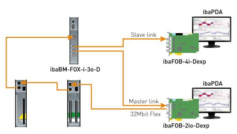
The fiber optic output of the last Flex device is connected to the input of an ibaBM-FOXi-3o-D device. One output of ibaBM-FOX-i-3o-D is connected to an input of the master ibaPDA, another output is connected to an input of the slave ibaPDA.
