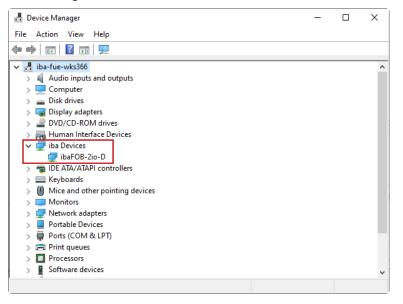
A node *iba Devices* must be displayed and below it the corresponding board (here *FOB-2io-D*).
