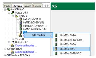
To configure the output signals, you must select the Outputs tab.
